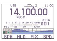
NOTE: If there is a lot of signal noise, turn the preamp OFF and the attenuator ON (p. 74) to reduce the input level and improve the readability of the scope.
